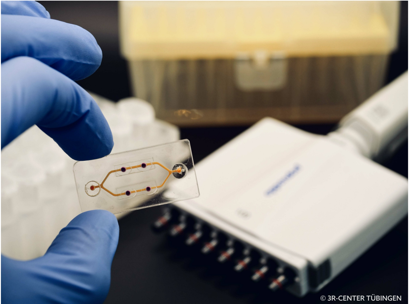
A model of a cervix has been developed on the Cervix-on-Chip. Substances are supplied and removed through the small channels. © 3R-Center Tübingen
