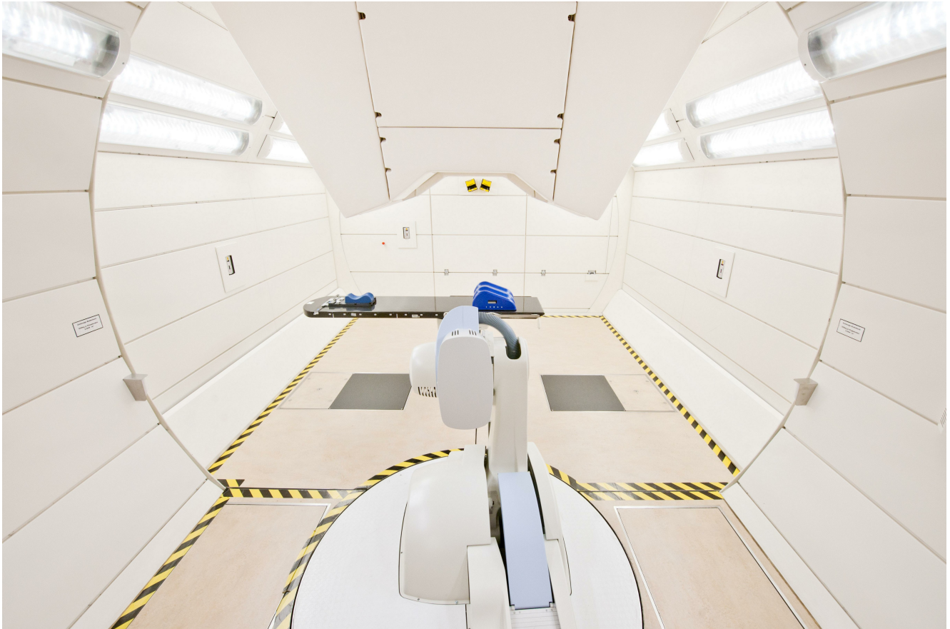
Radiotherapy room with rotatable (360°) radiation source, the so-called gantry. The ion beam can be directed onto the tumour from any direction. The HIT has two further treatment stations with fixed horizontal beam guidance.
