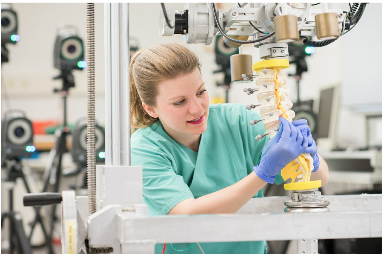
Doctoral student Laura Zengerle uses a plastic model to demonstrate how the spinal stress simulator works. © Elvira Eberhardt, Uni Ulm
