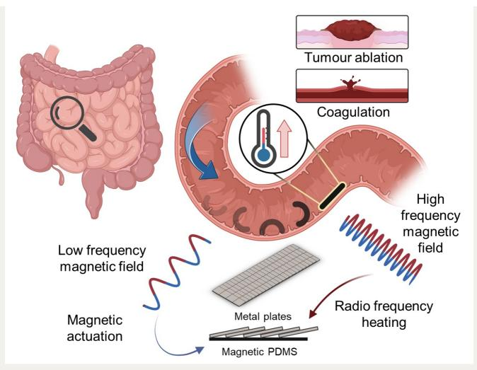
Schematic representation of how the wireless mini robot works in the small intestine. The device can be controlled using a low-frequency magnetic field; high frequencies cause the small aluminium plates to heat up, which can stop bleeding or destroy tumours, for example. Source: https://doi.org/10.1038/s41467-023-38689-x, Ren Hao Soon, CC BY 4.0 (https://creativecommons.org/licenses/by/4.0/)
