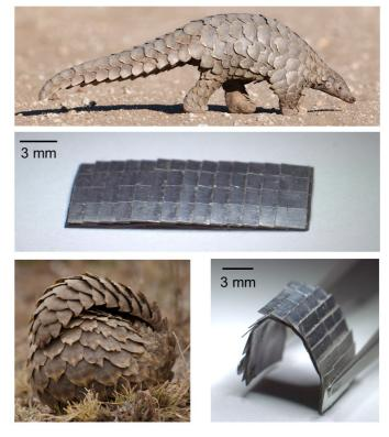
Based on the pangolin, which has armour consisting of individual overlapping hard keratin scales attached to the body, the new robot has a soft underside with a layer of overlapping, solid metal elements. This structure enables a high degree of flexibility. Source: https://doi.org/10.1038/s41467-023-38689-x, Ren Hao Soon, CC BY 4.0 (https://creativecommons.org/licenses/by/4.0/)
