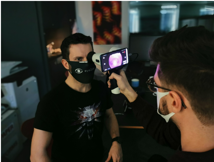
A retinal image taken with the help of a mobile system consisting of a funduscope and a smartphone. Dilating agents for a more complete view of the entire retina are not required. The eye2you AI provides understandable information about the probable disease.
