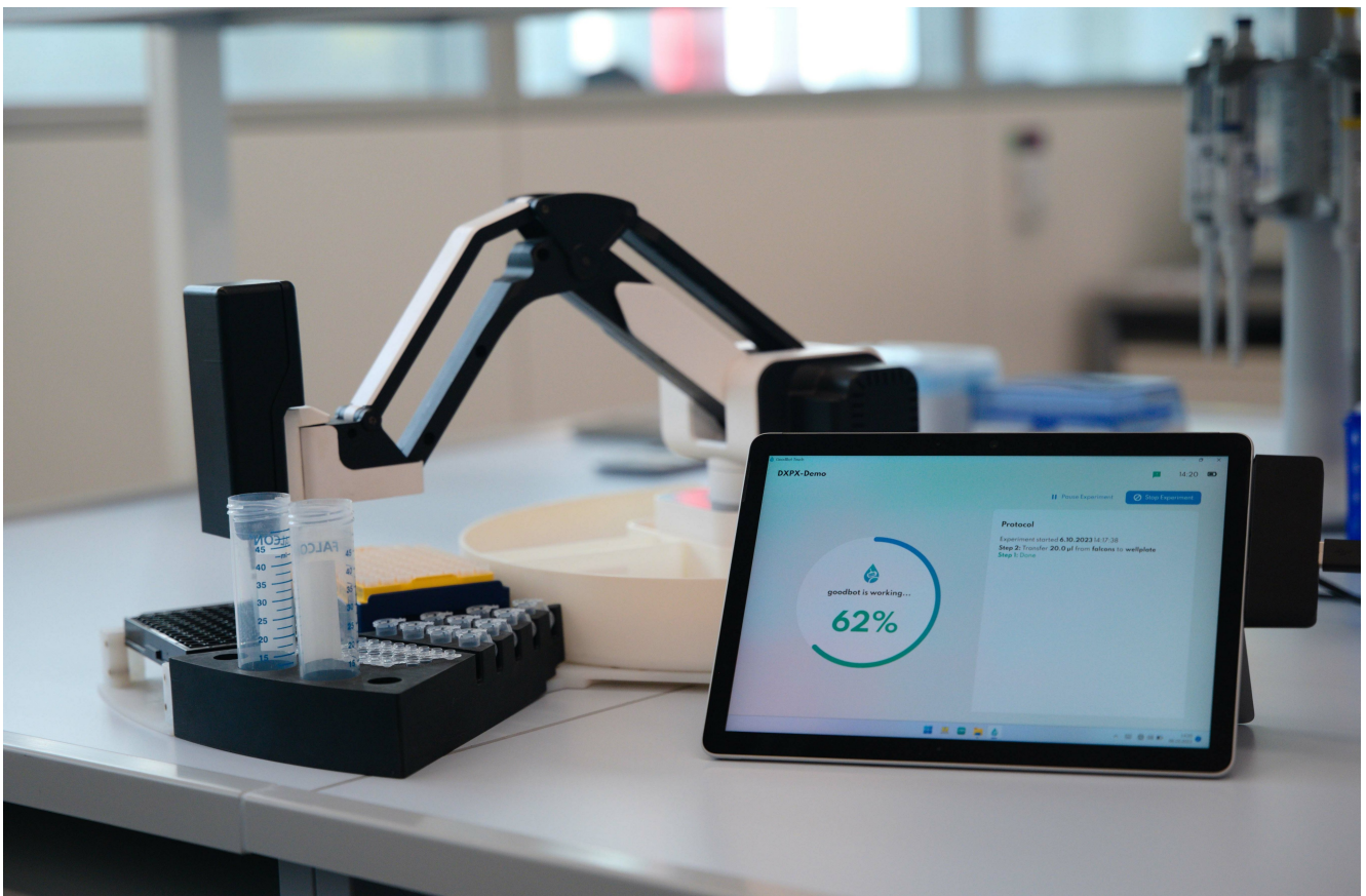
Vessels can be used in variable sizes from 1 µl to 1 ml. The goodBot software is also extremely user-friendly and requires no additional training. © goodBot GmbH
