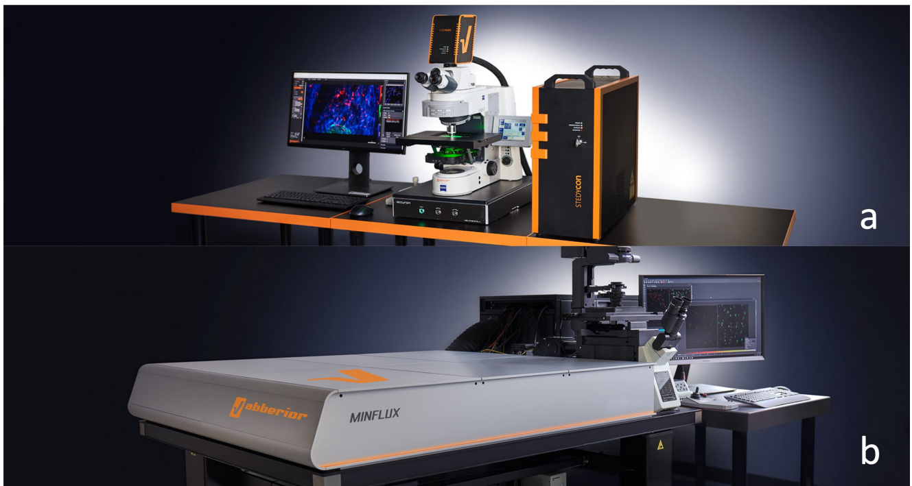
The shoebox-sized STEDYCON (image a) expands all conventional systems via a free camera access into a confocal microscope as well as a high-resolution STED nanoscope. MINFLUX (image b) is the world's most powerful light microscope.
