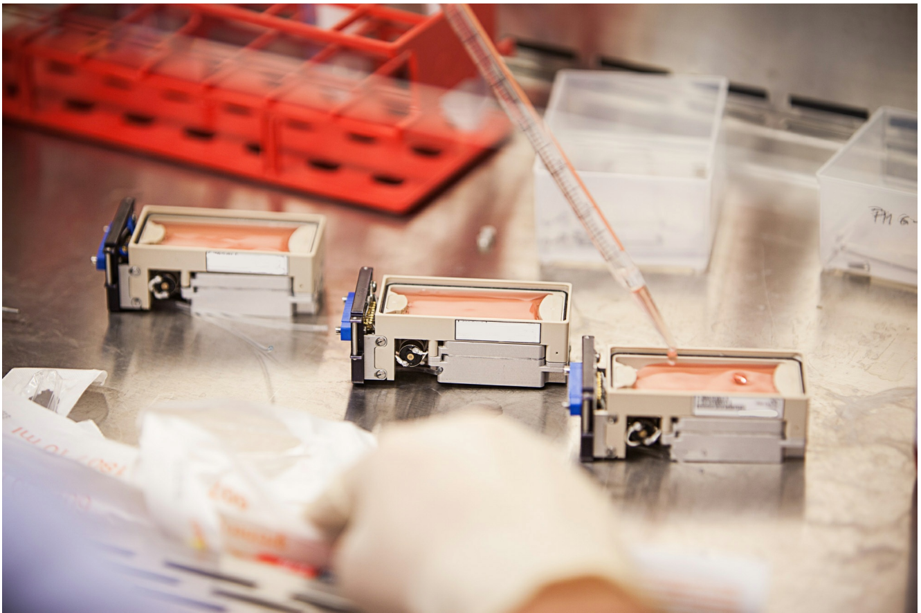
Miniature cell cultures: the research chamber with pump and tanks for the nutrient and fixative solution for the cells is roughly the size of a smartphone. © yuri GmbH
